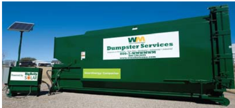
Type of solar compactor on site
